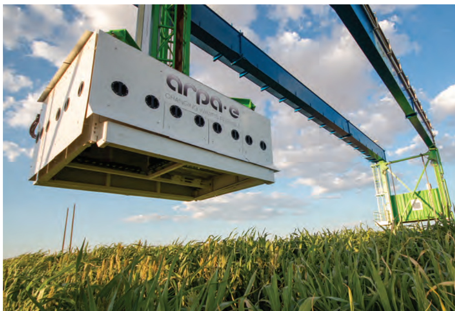
▲ High-throughput phenotyping gantry scans sorghum plots with precision cameras to accelerate crop improvement.
