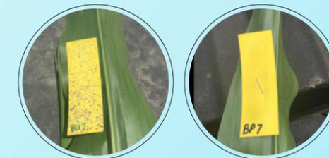
+ Comparison of coverage on the bottom side of corn leaves: 360 UNDERCOVER (left) and aerial application (right)
